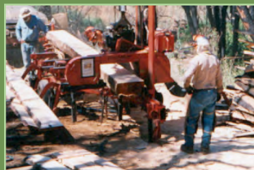
Milling trees killed in the fire for construction lumber. Nexus -- "waste" -- Materials
